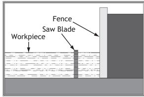
Figure 29. Example of a through cut.
